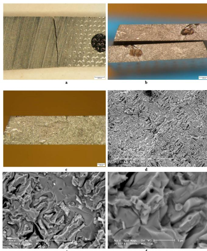
Fig. 10. Fractographic aspects of CoCrMoTi5 surfaces after tensile test: a, b, c- stereomicroscope images; d, e, f- cross sectional SEM images
