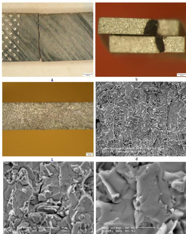
Fig. 8. Fractographic aspects of CoCrMoTiZr surfaces after tensile test: a, b, c- stereomicroscope images; d, e, f- cross sectional SEM images
