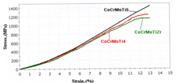
Fig. 7. Stress vs. Strain curves of cobalt alloys at bending test
