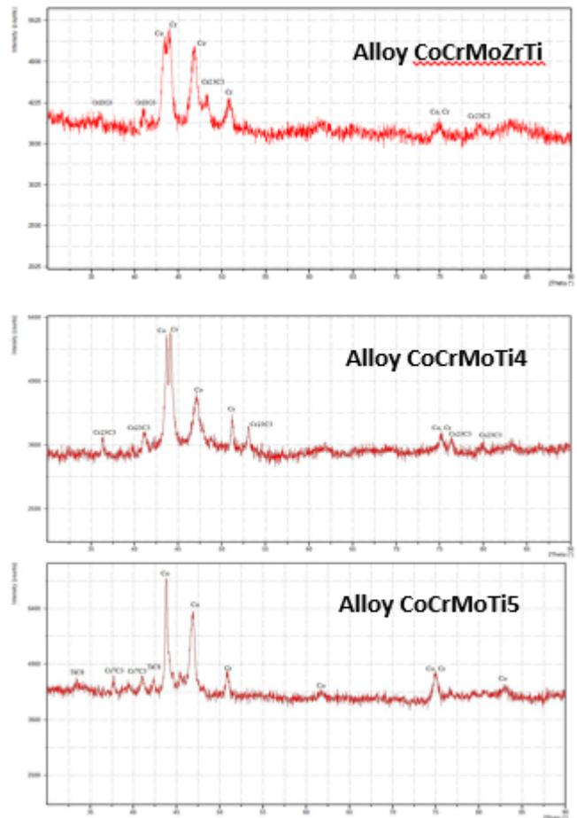
Fig. 5 X-Ray diffraction patterns of the cobalt alloys
