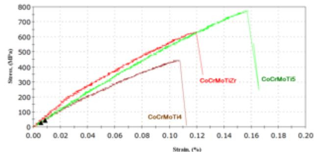
Fig. 6. Stress vs. Strain curves of cobalt alloys at tensile test
