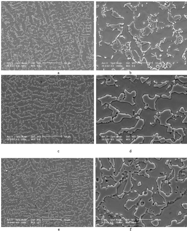
Fig. 4. SEM images of the cobalt alloys (electrolytic attack  $\text{HCl} + \text{HNO}_3 + \text{H}_2\text{O}_2$ ): a, b- CoCrMoTiZr alloy, c, d- CoCrMoTi4 alloy, e, f- CoCrMoTi5 alloy
