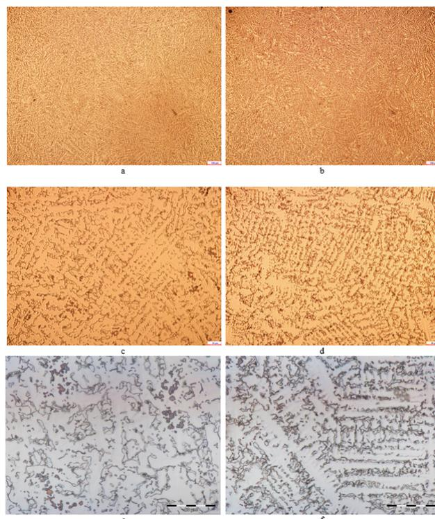
Fig. 1. Structural aspect of the CoCrMoTiZr alloy (Electrolytic attack HCl+HNO<sub>3</sub>+H<sub>2</sub>O<sub>2</sub>): a, c, e- central field; b, d, f- edge zone
